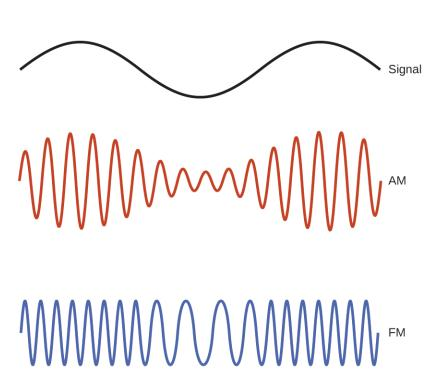
Figure 6.5 This schematic depicts how amplitude modulation (AM) and frequency modulation (FM) can be used to transmit a radio wave.
