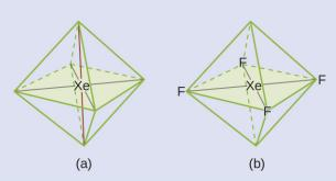
Figure 7.25 (a)  $XeF_4$  adopts an octahedral arrangement with two lone pairs (red lines) and four bonds in the electron-pair geometry. (b) The molecular structure is square planar with the lone pairs directly across from one another.
