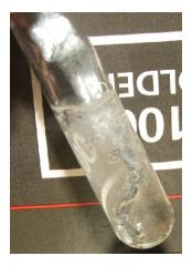
**Figure 18.7** Zinc is an active metal. It dissolves in hydrochloric acid, forming a solution of colorless Zn<sup>2+</sup> ions, Cl<sup>-</sup>ions, and hydrogen gas.
