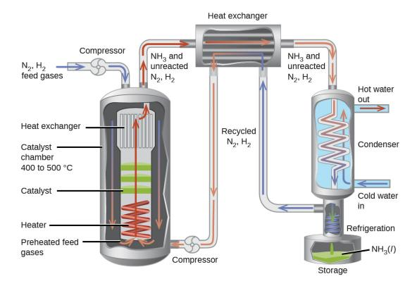
**Figure 13.10** Commercial production of ammonia requires heavy equipment to handle the high temperatures and pressures required. This schematic outlines the design of an ammonia plant.
