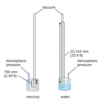
Figure 9.4 In a barometer, the height, h, of the column of liquid is used as a measurement of the air pressure. Using very dense liquid mercury (left) permits the construction of reasonably sized barometers, whereas using water (right) would require a barometer more than 30 feet tall.
