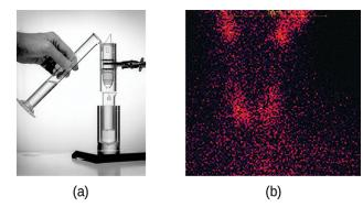
Figure 21.25 (a) The first Tc-99m generator (circa 1958) is used to separate Tc-99 from Mo-99. The  ${\rm MoO_4}^{2-}$  is retained by the matrix in the column, whereas the  ${\rm TcO_4}^-$  passes through and is collected. (b) Tc-99 was used in this scan of the neck of a patient with Grave's disease. The scan shows the location of high concentrations of Tc-99. (credit a: modification of work by the Department of Energy; credit b: modification of work by "MBq"/Wikimedia Commons)
