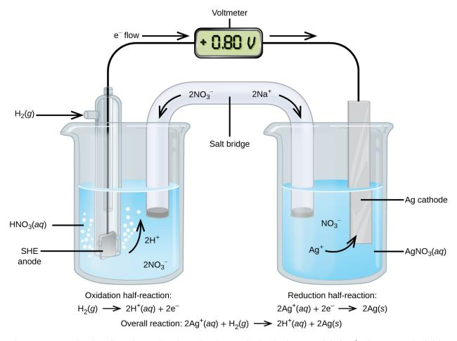
Figure 17.8 A galvanic cell can be used to determine the standard reduction potential of  $Ag^+$ . The SHE on the left is the anode and assigned a standard reduction potential of zero.
