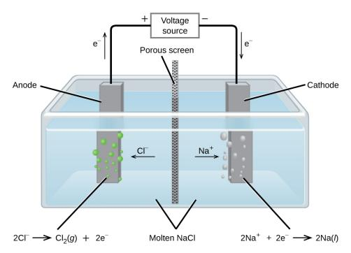
**Figure 17.19** Passing an electric current through molten sodium chloride decomposes the material into sodium metal and chlorine gas. Care must be taken to keep the products separated to prevent the spontaneous formation of sodium chloride.
