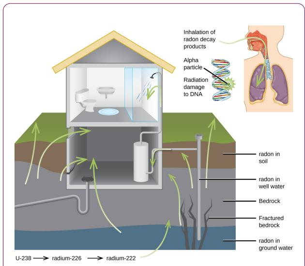
**Figure 21.34** Radon-222 seeps into houses and other buildings from rocks that contain uranium-238, a radon emitter. The radon enters through cracks in concrete foundations and basement floors, stone or porous cinderblock foundations, and openings for water and gas pipes.
