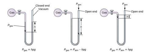
Figure 9.5 A manometer can be used to measure the pressure of a gas. The (difference in) height between the liquid levels (h) is a measure of the pressure. Mercury is usually used because of its large density.
