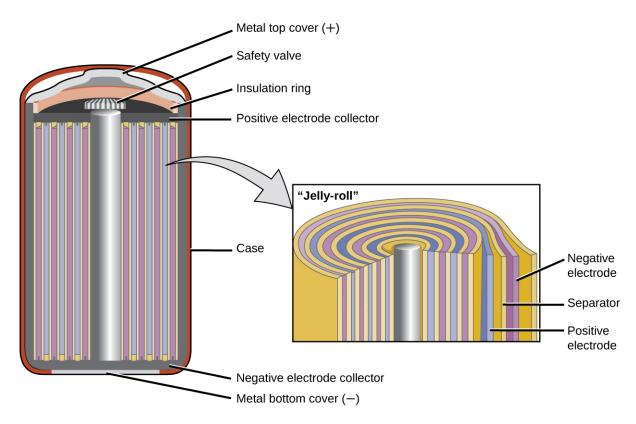
**Figure 17.12** NiCd batteries use a "jelly-roll" design that significantly increases the amount of current the battery can deliver as compared to a similar-sized alkaline battery.
