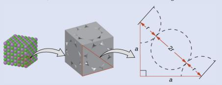
Drawing a right triangle on the face of the unit cell, we see that the length of the diagonal is equal to four chloride radii (one radius from each corner chloride and one diameter—which equals two radii—from the chloride ion in the center of the face), so d = 4r. From the Pythagorean theorem, we have:
