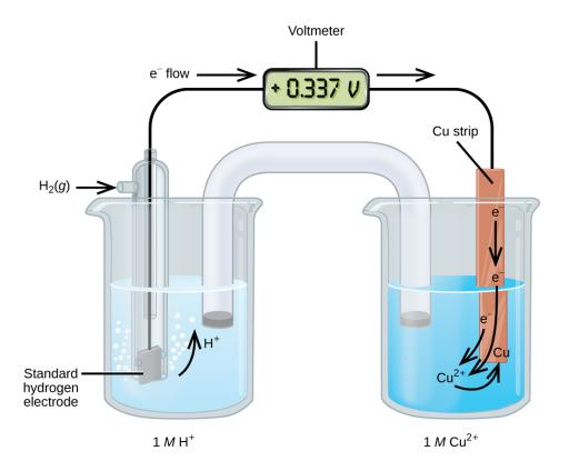
Figure 17.7 A galvanic cell can be used to determine the standard reduction potential of Cu<sup>2+</sup>.
