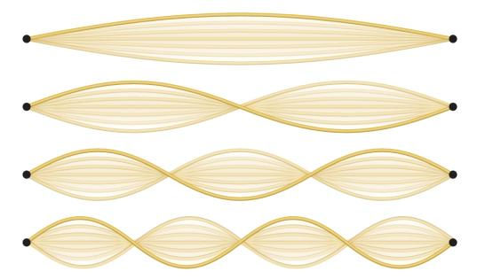
**Figure 6.7** A vibrating string shows some one-dimensional standing waves. Since the two end points of the string are held fixed, only waves having an integer number of half-wavelengths can form. The points on the string between the end points that are not moving are called the nodes.
