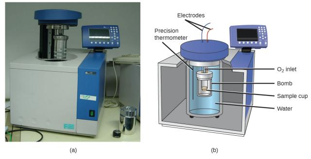
Figure 5.17 (a) A bomb calorimeter is used to measure heat produced by reactions involving gaseous reactants or products, such as combustion. (b) The reactants are contained in the gas-tight "bomb," which is submerged in water and surrounded by insulating materials. (credit a: modification of work by "Harbor1"/Wikimedia commons)
