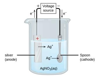
**Figure 17.21** The spoon, which is made of an inexpensive metal, is connected to the negative terminal of the voltage source and acts as the cathode. The anode is a silver electrode. Both electrodes are immersed in a silver nitrate solution. When a steady current is passed through the solution, the net result is that silver metal is removed from the anode and deposited on the cathode.
