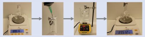
**Figure 9.19** When the volatile liquid in the flask is heated past its boiling point, it becomes gas and drives air out of the flask. At  $t_l \longrightarrow g^*$  the flask is filled with volatile liquid gas at the same pressure as the atmosphere. If the flask is then cooled to room temperature, the gas condenses and the mass of the gas that filled the flask, and is now liquid, can be measured. (credit: modification of work by Mark Ott)
