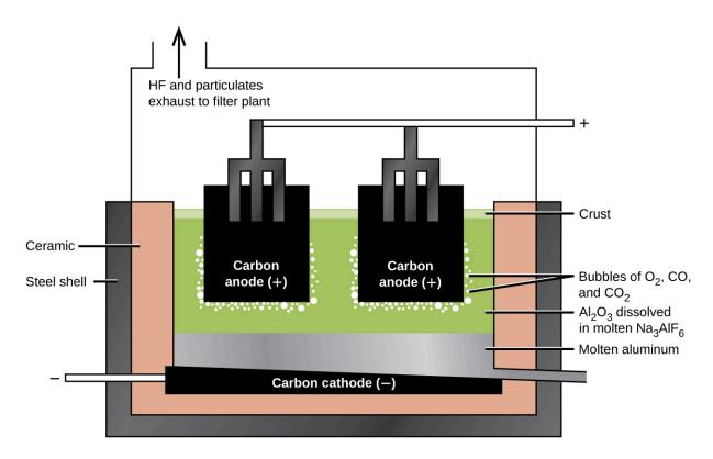
**Figure 18.11** An electrolytic cell is used for the production of aluminum. The electrolysis of a solution of cryolite and calcium fluoride results in aluminum metal at the cathode, and oxygen, carbon monoxide, and carbon dioxide at the anode.
