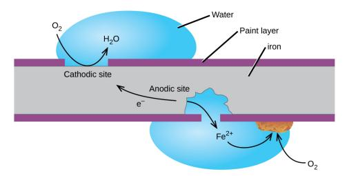
**Figure 17.17** Once the paint is scratched on a painted iron surface, corrosion occurs and rust begins to form. The speed of the spontaneous reaction is increased in the presence of electrolytes, such as the sodium chloride used on roads to melt ice and snow or in salt water.
