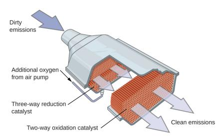
**Figure 12.27** A catalytic converter allows for the combustion of all carbon-containing compounds to carbon dioxide, while at the same time reducing the output of nitrogen oxide and other pollutants in emissions from gasoline-burning engines.
