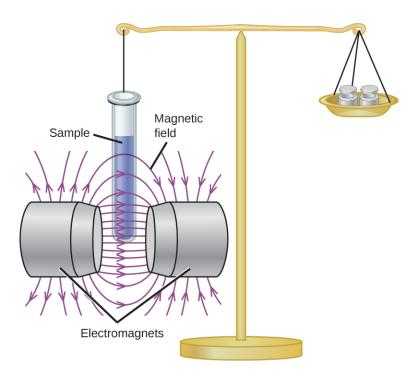
**Figure 8.27** A Gouy balance compares the mass of a sample in the presence of a magnetic field with the mass with the electromagnet turned off to determine the number of unpaired electrons in a sample.
