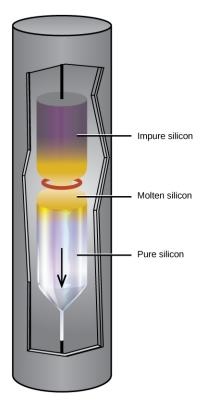
Figure 18.14 A zone-refining apparatus used to purify silicon.
