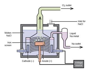
**Figure 18.10** Pure sodium metal is isolated by electrolysis of molten sodium chloride using a Downs cell. It is not possible to isolate sodium by electrolysis of aqueous solutions of sodium salts because hydrogen ions are more easily reduced than are sodium ions; as a result, hydrogen gas forms at the cathode instead of the desired sodium metal. The high temperature required to melt NaCl means that liquid sodium metal forms.
