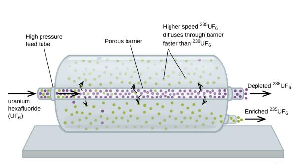
Figure 9.30 In a diffuser, gaseous UF<sub>6</sub> is pumped through a porous barrier, which partially separates  $^{235}$ UF<sub>6</sub> from  $^{238}$ UF<sub>6</sub> The UF<sub>6</sub> must pass through many large diffuser units to achieve sufficient enrichment in  $^{235}$ U.
