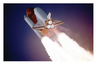
Figure 18.28 Before the fleet's retirement in 2011, liquid hydrogen and liquid oxygen were used in the three main engines of a space shuttle. Two compartments in the large tank held these liquids until the shuttle was launched. (credit: "reynermedia"/Flickr)
