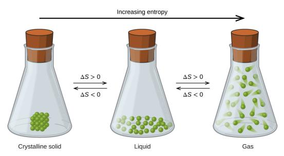
**Figure 16.10** The entropy of a substance increases ( $\Delta S > 0$ ) as it transforms from a relatively ordered solid, to a less-ordered liquid, and then to a still less-ordered gas. The entropy decreases ( $\Delta S < 0$ ) as the substance transforms from a gas to a liquid and then to a solid.
