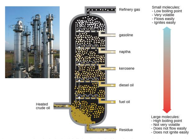
Figure 20.6 In a column for the fractional distillation of crude oil, oil heated to about 425 °C in the furnace vaporizes when it enters the base of the tower. The vapors rise through bubble caps in a series of trays in the tower. As the vapors gradually cool, fractions of higher, then of lower, boiling points condense to liquids and are drawn off. (credit left: modification of work by Luigi Chiesa)
