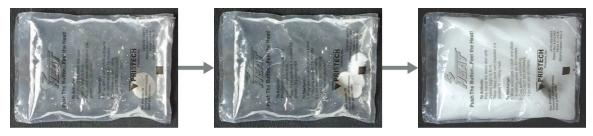
Figure 5.15 Chemical hand warmers produce heat that warms your hand on a cold day. In this one, you can see the metal disc that initiates the exothermic precipitation reaction. (credit: modification of work by Science Buddies TV/YouTube)
