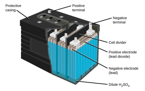
**Figure 17.14** The lead acid battery in your automobile consists of six cells connected in series to give 12 V. Their low cost and high current output makes these excellent candidates for providing power for automobile starter motors.
