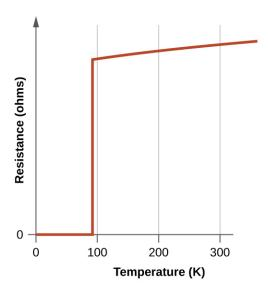
Figure 19.10 The resistance of the high-temperature superconductor YBa<sub>2</sub>Cu<sub>3</sub>O<sub>7</sub> varies with temperature. Note how the resistance falls to zero below 92 K, when the substance becomes superconducting.
