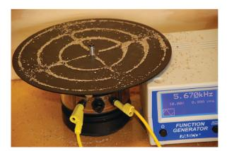
**Figure 6.8** Two-dimensional standing waves can be visualized on a vibrating surface. The surface has been sprinkled with a powder that collects near the nodal lines. There are two types of nodes visible: radial nodes (circles) and angular nodes (radii).
