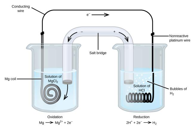
**Figure 17.5** The oxidation of magnesium to magnesium ion occurs in the beaker on the left side in this apparatus; the reduction of hydrogen ions to hydrogen occurs in the beaker on the right. A nonreactive, or inert, platinum wire allows electrons from the left beaker to move into the right beaker. The overall reaction is:
