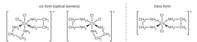
Figure 19.24 Three isomeric forms of  $[Co(en)_2Cl_2]^+$  exist. The *trans* isomer, formed when the chlorines are positioned at a 180° angle, has very different properties from the *cis* isomers. The mirror images of the *cis* isomer form a pair of optical isomers, which have identical behavior except when reacting with other enantiomers.
