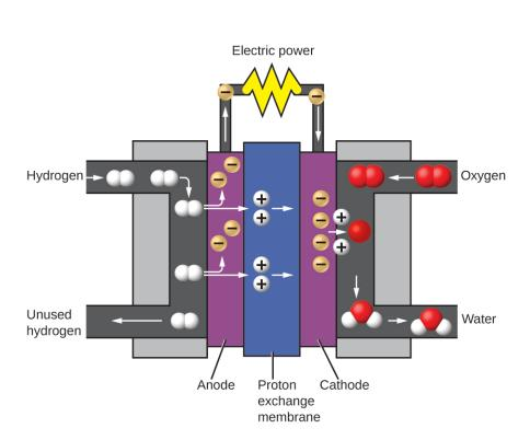
**Figure 1.16** A fuel cell generates electrical energy from hydrogen and oxygen via an electrochemical process and produces only water as the waste product.
