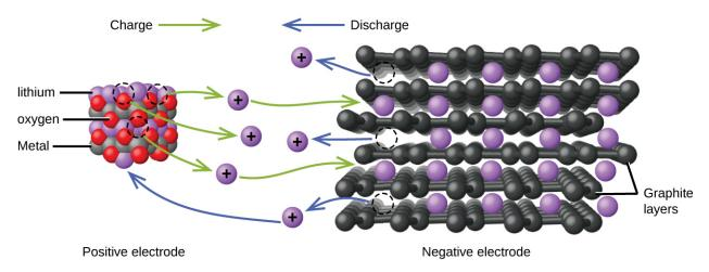
Figure 17.13 In a lithium ion battery, charge flows between the electrodes as the lithium ions move between the anode and cathode.
