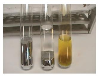
Figure 18.8 From left to right: Hg(I), Hg + concentrated HCl, Hg + concentrated HNO<sub>3</sub>. (credit: Sahar Atwa)
